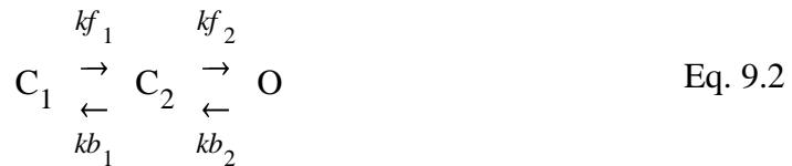
The closed states are  $C_1$  and  $C_2$ , the open state is  $O$ , and the rates of the forward and backward state transitions are calculated in terms of the equilibrium constants and time
