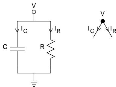
Fig. 3.4. Left: Schematic diagram of a simple parallel RC circuit, which has only one node at which potential is unknown. Right: Node diagram indicating the flow of current away from this single node.
