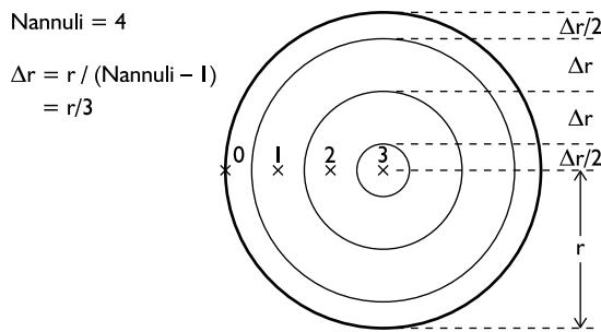
Figure 9.9. Diagram of the concentric shells used to model radial diffusion. The  $x$  mark the radial distances at which concentration will be second order correct in space.
