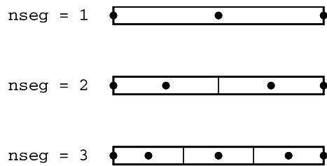
Figure 5.3. Each section has a discretization parameter `nseg` that governs the number of internal nodes (black dots inside the section) at which membrane potential is computed. The thin lines mark conceptual boundaries between adjacent segments.
