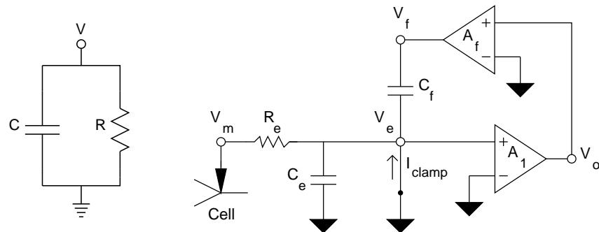
Fig. 3.3. Left: A simple parallel RC circuit. Right: Circuit for recording from a cell while passing current through the same electrode. Amplifier  $A_f$  and capacitor  $C_f$  are used to compensate for the electrode capacitance  $C_e$ .
