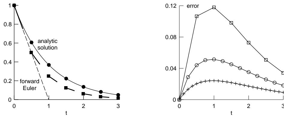
Figure 4.3. Left: analytic solution to Eq. 4.19 (solid line with circles) and results of the forward Euler method (squares) for  $V(0) = 1$ ,  $k = 1/\text{s}$ , and  $\Delta t = 0.5 \text{ s}$  (modified from (Hines and Carnevale 1997)). Right: absolute error of the forward Euler method with  $\Delta t = 0.5$  (squares), 0.25 (circles), and 0.125 s (+).
