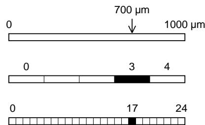
Figure 5.4. Boxed in by compartments. Top: Conceptual model of an unbranched axon 1000  $\mu\text{m}$  long. We are interested in membrane potential at a point 700  $\mu\text{m}$  from its left end. Middle and bottom: The index of the compartment that corresponds to the location of interest depends on how many compartments there are.
