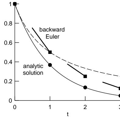
Figure 4.5. Comparison of analytic solution to Eq. 4.19 (solid line with circles) with results from the backward Euler method (Eq. 4.25, squares) for  $V(0) = 1$ ,  $k = 1/s$ , and  $\Delta t = 1$  s. At the end of each step, the slope at the new value (heavy lines) points back to the beginning of the step. The dashed line shows the voltage after the first time step as a function of  $\Delta t$ . Modified from (Hines and Carnevale 1997).
