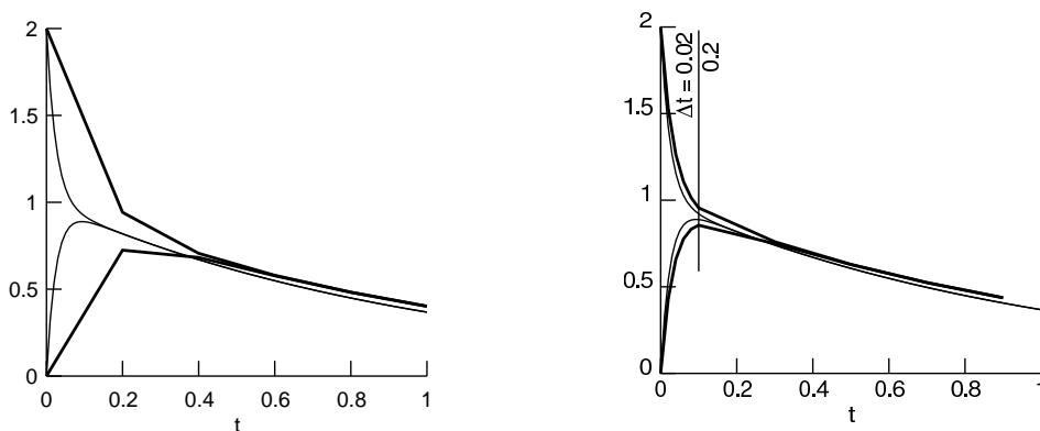
Figure 4.6. Simulation of the two compartment model of Fig. 4.4 using the backward Euler method. Left:  $\Delta t = 0.2$  s, much larger than the fast time constant. Right:  $\Delta t$  was initially 0.02 s, small enough to follow the first time constant closely. After 0.1 s,  $\Delta t$  increased to 0.2 s but the solution remained stable. Thin lines are analytic solution, thick lines are backward Euler solution.
